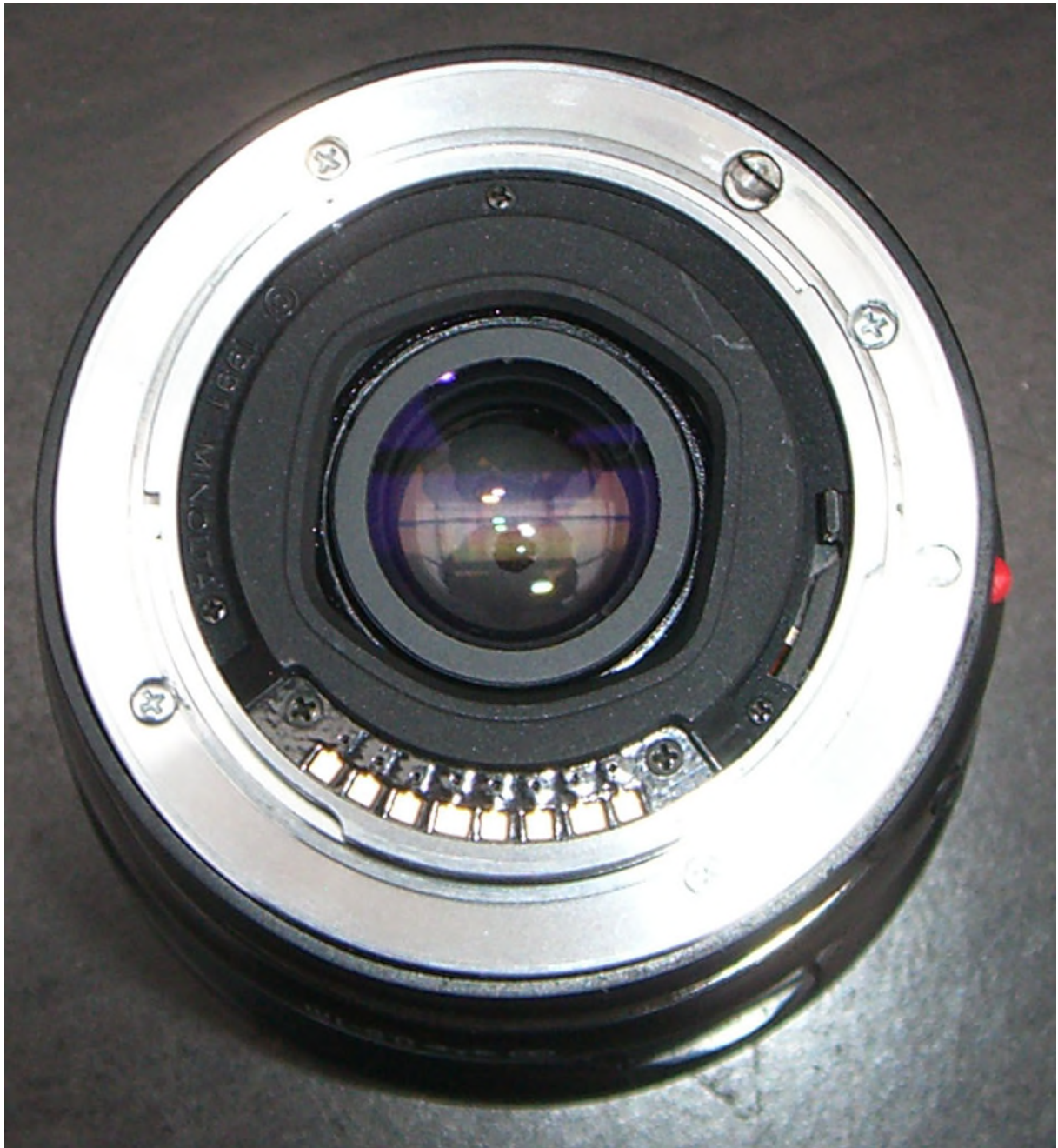
Minolta AF bayonet >> Sony A-mount bayonet (Sony Alpha Axx and Axxx, x=number), inner diameter 45 mm, outer diameter 47mm (without bay.teeth)
