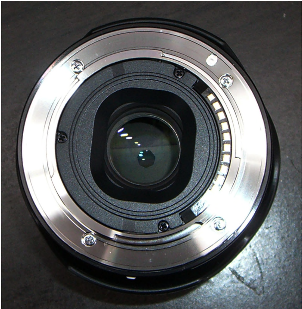
Sony E-mount bayonet, new for direct-sensor, mirrorless camera types (NEX, Ax and Axxxx, x=number), inner diameter 41,5mm, outer d. 48mm (without bay.teeth), objective types: E (APS-C), FE (Full Frame 35mm)
